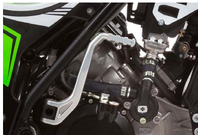
Engine kick-start pedal joints
