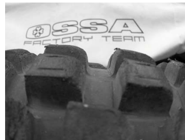
Tyre in bad working condition
