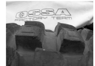
Tyre in bad working condition
